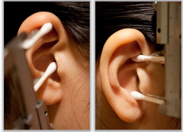
FIG. 10. (Color online) Practical measurement of pinna anthropometric distances for estimation of Cavum-Fossa and Cavum-Cymba normal mode frequencies, using cotton buds attached to a pair of calipers, on pinna "fAr" [the same pinna depicted in Figs. 4(a) and 7(a)]. Left panel: measurement of the distance d_{1-17} between ear-canal entrance and helix rim, for estimation of F_{\text{cav-fos}} using Eq. (3). Right panel: measurement of the vertical distance d_{4-12(\text{vert})} between concha floor and cymba anterior wall, for estimation of F_{\text{cav-cym}} using Eq. (8).
