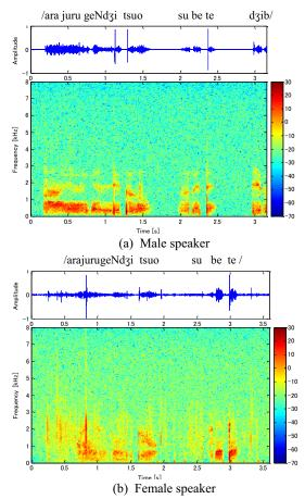
Figure 5: Waveform and spectrogram of NAM signals for (a) male and (b) female speaker recorded with soft-silicone type NAM microphone.
