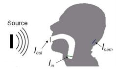
Figure 3: Geometry of simulated region including head, sound source, and receivers.
