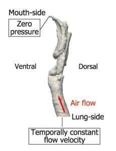
Figure 1: Sagittal view of vocal tract shape model. Air flows from lung-side to mouth-side. Temporally constant flow velocity given at lung-side boundary. Zero pressure given at mouth-side boundary.
