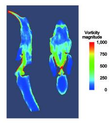
Figure 2: Instantaneous vorticity magnitude (in [1/s]) distributions on sagittal and coronal sections for NAM. Color bar ranges from 0 to 1,000.
