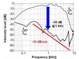
Figure 4: Vocal-tract transfer functions  $I_{in}/I_{out}$  and  $I_{nam}/I_{out}$ corresponds to sound intensity level observed at NAM microphone assuming sound radiating from mouth has flat frequency characteristics.
