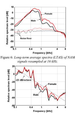
Figure 7: Long-term average spectra (LTAS) of underlying NAM signals by subtracting frequency responses of NAM microphone and amplifier from LTAS shown in Fig. 6.
